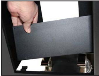
5. Remove Access panel to J-Box and Ballast.
